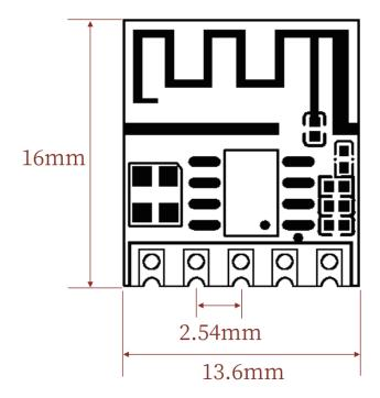
Component height+board thickness: 2.63mm
